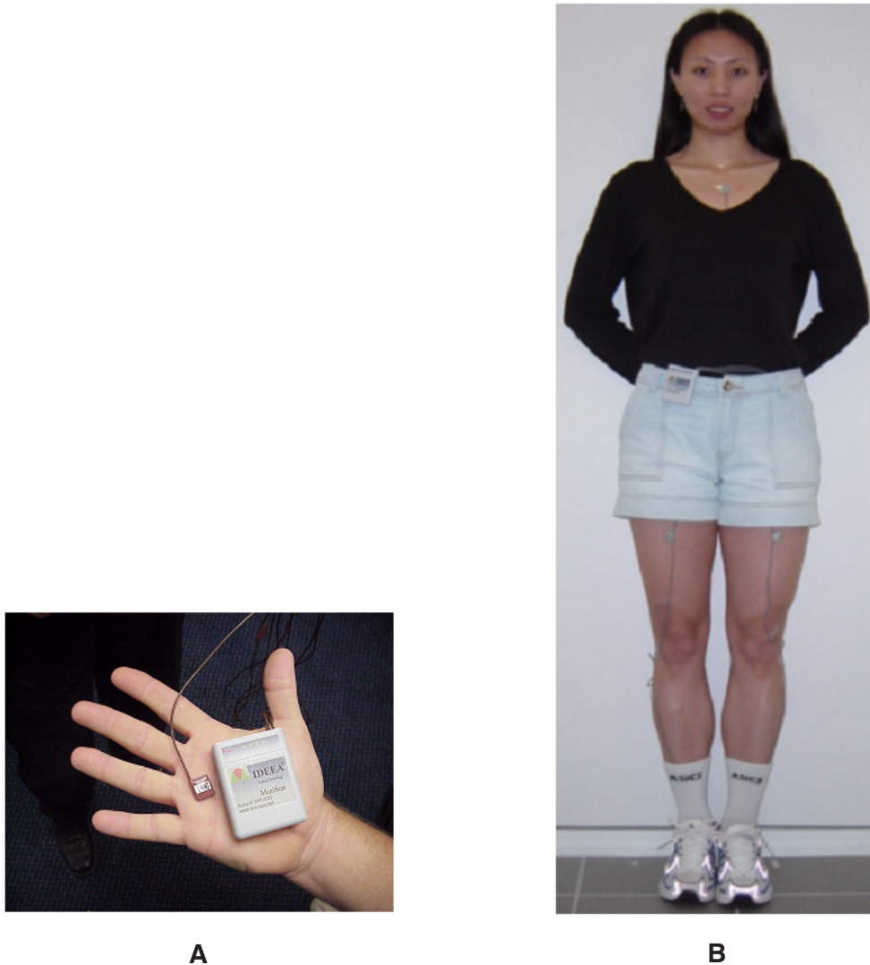
FIGURE 1. (A) The photo of PMA recording device with one sensor held by one hand. (B) Positions of sensors: a subject wearing the PMA recorder.
