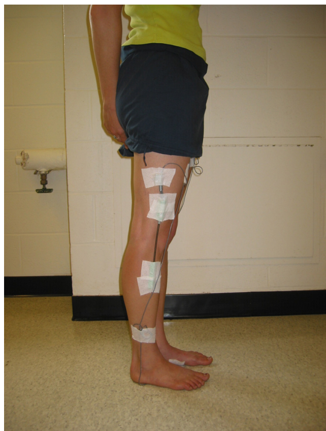
Figure 4 Photograph (side view) of the modified IDEEA system being worn by a patient.
