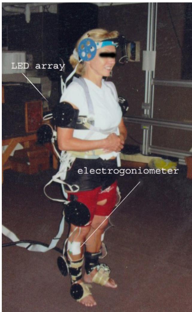
Figure 1 Photograph of a subject being tested in the MGH Biotion Laboratory with both the IDEEA system and LED arrays in place.
