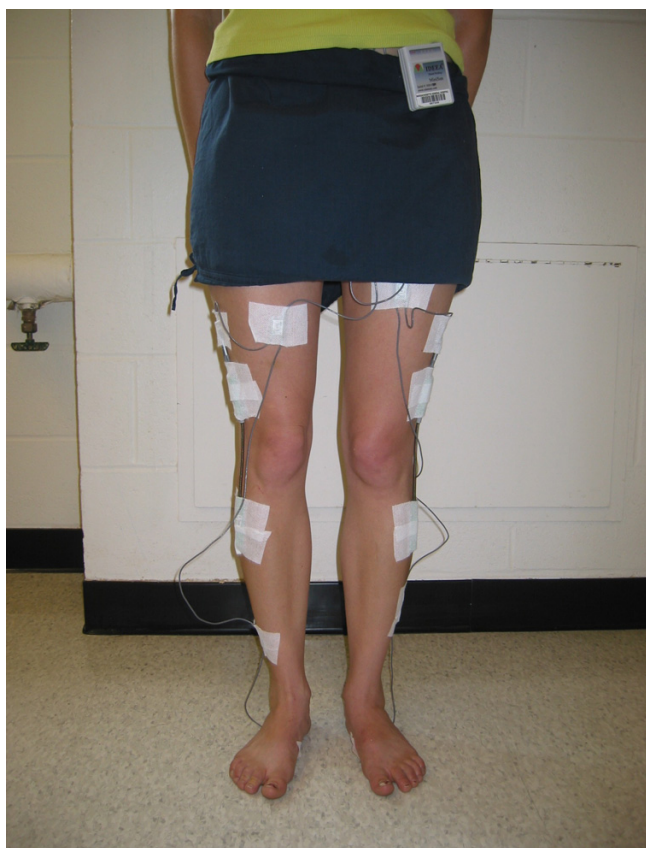
Figure 3 Photograph (front view) of the modified IDEEA system being worn by a patient.
